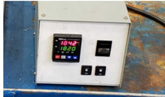
Test Heating Unit
